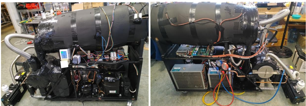
Fig. 4. Assembled machine for vacuum cold condensing
